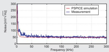
The measured output noise of the charge amplifier is about 50 nV/√Hz and fits to the simulated (PSPICE) noise performance results.
