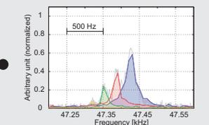
The frequency-shift can be corrected afterwards by determining the frequency-shift-function and suitable time-signal resampling. This method can improve mass resolution and also increase ion sensitivity.
