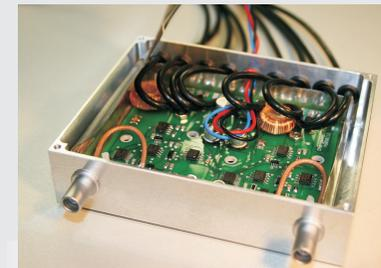
The charge amplifiers pick up the influence charges that are induced onto the inner cap-electrode by the oscillating ions inside the trap. This is done by a low noise JFET in combination with a low noise OP.
