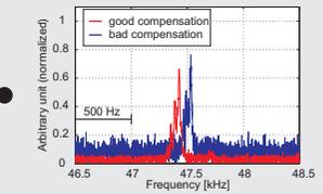
High ion densities result in space charges which cause a frequency-shift in the spectra.
