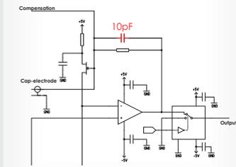
During the ion oscillation the ions induce an influence current in the charge amplifier. This current will be integrated by the capacitor in the feedback loop. As a result the electric charge stored in the capacitor corresponds to the charged particles inside the trap (e.g. the number of ions). Because of the Q-V-conversion characteristic of the capacitor we are able to compute the number of ions inside the trap by measuring the ion signal amplitude at the beginning of the ion transient:
