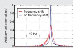
Stored ions inside the trap cause space charges which cause a frequency-shift over time. This will reduce mass resolution.
