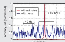
It is possible with the given noise level to detect down to 65 ions at low residual pressures (blue). The red curve shows the transient and spectra for a noise-free system.
