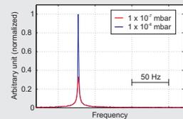
Simulations show that the residual pressure is an important factor for ion sensitivity. Because of more ion-residual gas-collisions the ion transient will be shorter and the energy in the signal is lower.
