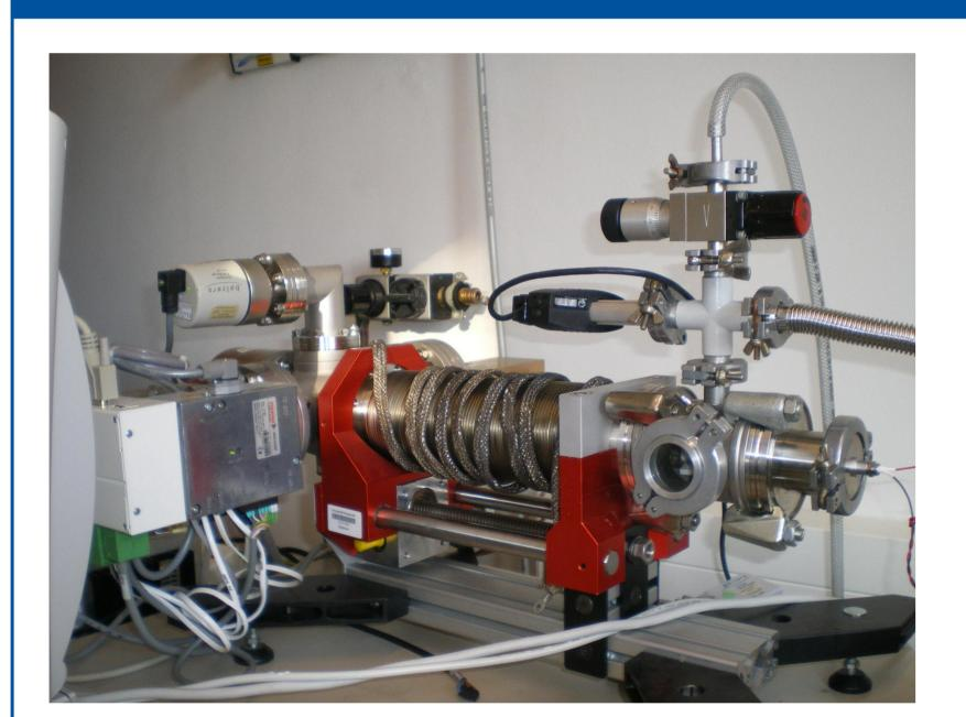
MS experimental set-up. Piezo plasma source (not visible) is located in the small vacuum chamber to the right.
