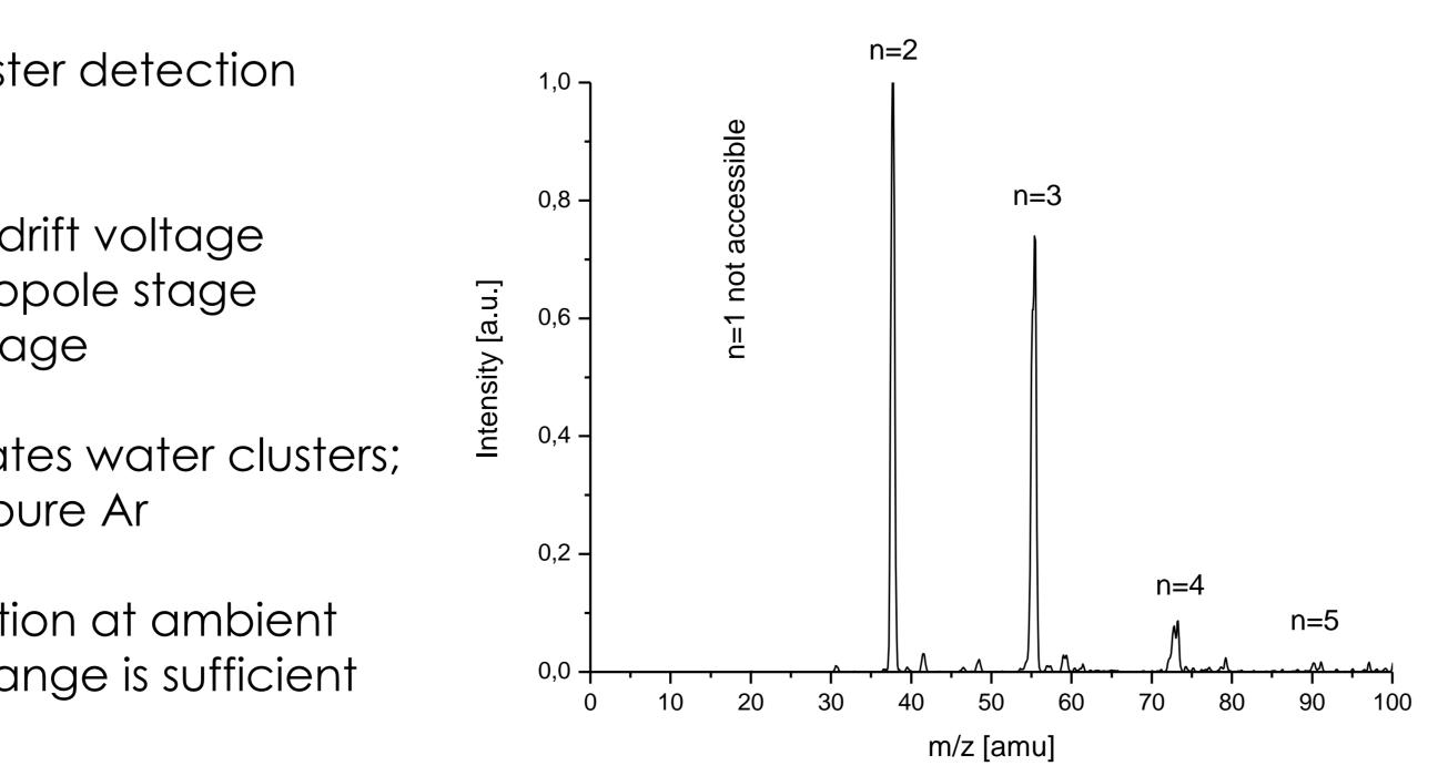
conditions: water admixture by exposing Ar gas to liquid water reservoir upstream from DBD, then freezing the reservoir
